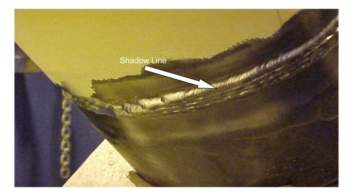
*Stringer Bead Technique:* Run the puddle edge along the line formed where the light from the arc disappears under the first pass and continue with each following pass. This technique can be used on pipe in the 2g, 5g, and 6g positions.
