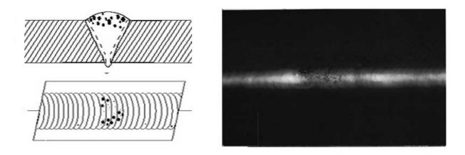
**Slag inclusions** are nonmetallic solid material entrapped in weld metal or between weld and base metal. In a radiograph, dark, jagged asymmetrical shapes within the weld or along the weld joint areas are indicative of slag inclusions.
