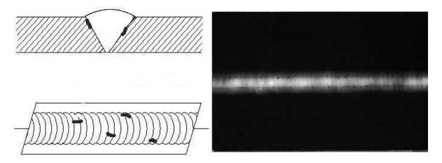
**Internal concavity or suck back** is a condition where the weld metal has contracted as it cools and has been drawn up into the root of the weld. On a radiograph it looks similar to a lack of penetration but the line has irregular edges and it is often quite wide in the center of the weld image.
