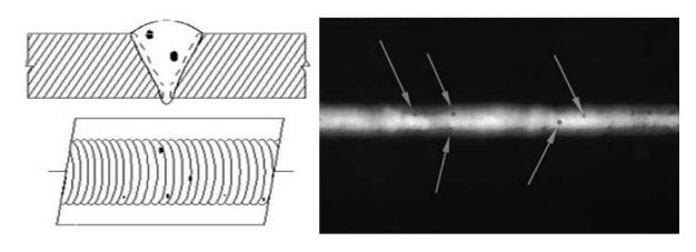
**Cluster porosity** is caused when flux coated electrodes are contaminated with moisture. The moisture turns into a gas when heated and becomes trapped in the weld during the welding process. Cluster porosity appears just like regular porosity in the radiograph but the indications will be grouped close together.
