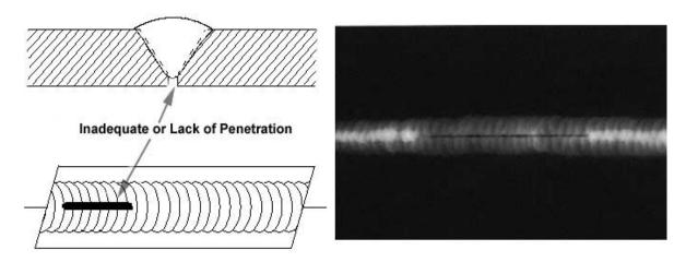
**Incomplete fusion** is a condition where the weld filler metal does not properly fuse with the base metal. Appearance on radiograph: usually appears as a dark line or lines oriented in the direction of the weld seam along the weld preparation or joining area.
