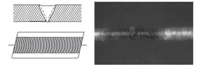
**Excess weld reinforcement** is an area of a weld that has weld metal added in excess of that specified by engineering drawings and codes. The appearance on a radiograph is a localized, lighter area in the weld. A visual inspection will easily determine if the weld reinforcement is in excess of that specified by the engineering requirements.
