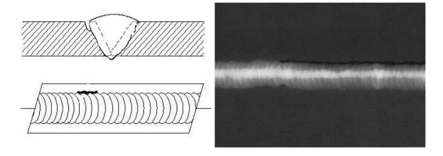
Offset or mismatch are terms associated with a condition where two pieces being welded together are not properly aligned. The radiographic image shows a noticeable difference in density between the two pieces. The difference in density is caused by the difference in material thickness. The dark, straight line is caused by the failure of the weld metal to fuse with the land area.
