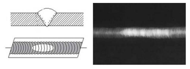
**Cracks** can be detected in a radiograph only when they are propagating in a direction that produces a change in thickness that is parallel to the x-ray beam. Cracks will appear as jagged and often very faint irregular lines. Cracks can sometimes appear as "tails" on inclusions or porosity.
