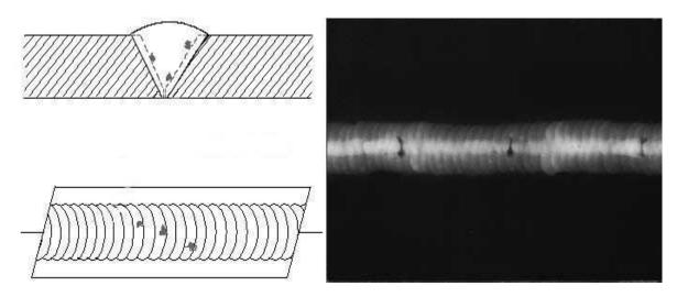
**Incomplete penetration (IP) or lack of penetration (LOP)** occurs when the weld metal fails to penetrate the joint. It is one of the most objectionable weld discontinuities. Lack of penetration allows a natural stress riser from which a crack may propagate. The appearance on a radiograph is a dark area with well-defined, straight edges that follows the land or root face down the center of the weldment.
