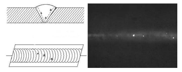
**Oxide inclusions** are usually visible on the surface of material being welded (especially aluminum). Oxide inclusions are less dense than the surrounding material and, therefore, appear as dark irregularly shaped discontinuities in the radiograph.
